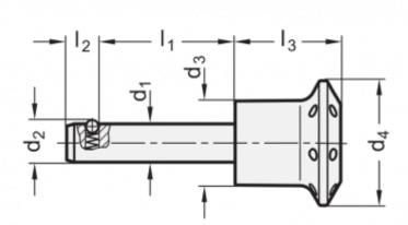
Axial grasping power on pins N = 15Bore for pin D12 = 8
